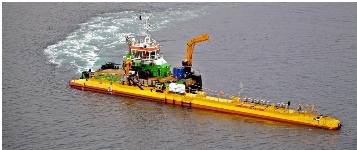
ORBITAL MARINEPOWER'S "ORBITAL 02" 2MW TIDEVANNSTURBIN. FOTO: ORKNEY.COM.
