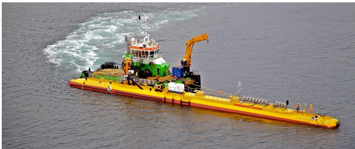
ORBITAL MARINEPOWER'S "ORBITAL 02" 2MW TIDEVANNSTURBIN. FOTO: ORKNEY.COM.
